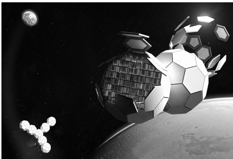
Figure 13 The modular and self-assembly structure of TESSERAE. Source: Artist Rendering of TESSERAE by TU Dortmund – MIT Media Lab.
